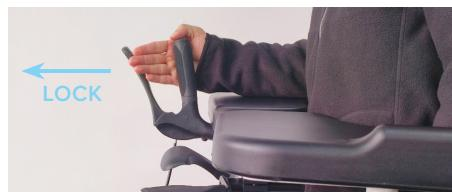
**TO UNLOCK THE BRAKES** Pull the brake handles backwards until they release.
