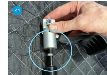
4.2 Remove the locking bolt set that is screwed into the bracket in the middle of the base frame. Insert the bottom of the height adjustment gas strut into the bracket and secure it with the locking nut kit, using a 6mm Allen key.
