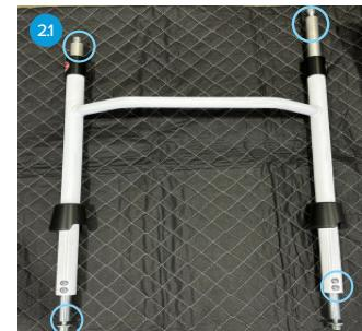
2.2 Attach the upright frame to the base frame by securing the walker with the M12 bolts and washer previously removed (from the bottom of the upright frame), inserting them through the bottom of the base frame, and tightening them using the 10mm Allen key.
