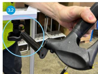
3.3 Secure them in place by tightening the locking levers located under the brake handles by hand.
